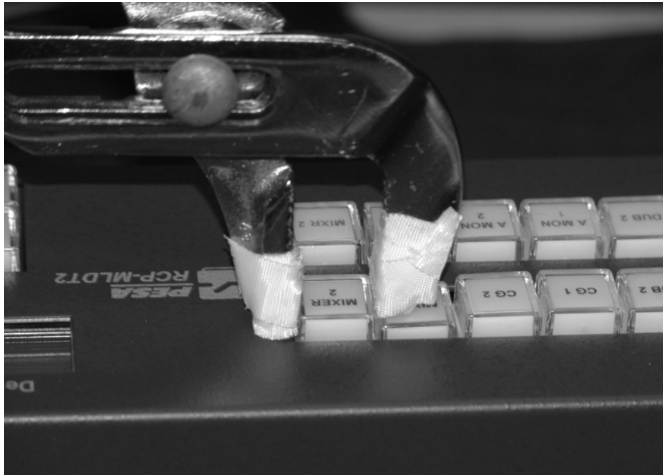
Figure 1-2 Grasp Lateral Edges of Switch Cap with Wrapped Pliers
