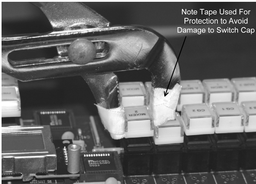
Figure 1-3 Panel Shown with Front Cover Removed for Better Access
