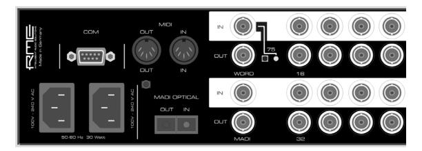
**IEC receptacle** for power connection. The specially developed, internal hi-performance switch mode power supply makes the ADI-6432 operate in the range of 100V to 240V AC. It is short-circuit-proof, has an integrated line-filter, is fully regulated against voltage fluctuations, and suppresses mains interference.
