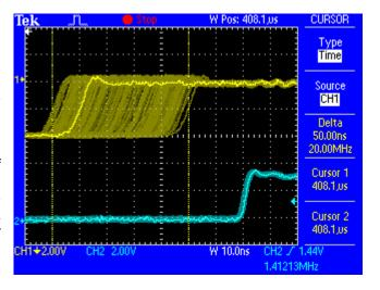
The cleaned and jitter-freed signal can be used as reference clock for any application, without any problem. The signal processed by SteadyClock is of course not only used internally, but also available at the ADI-6432's word clock output. It is also used to clock the digital outputs MADI and AES.
