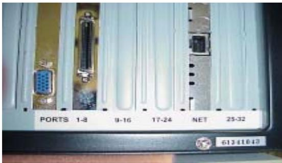
2. Interconnect one or more intercom audio ports between the intercom systems. These ports will be used for trunking communication only. Figure 10 and 11 indicate the specific cable wiring diagrams.
