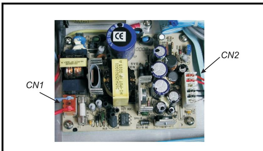
3. Remove the **four (4) placement screws** and remove the power supply.
