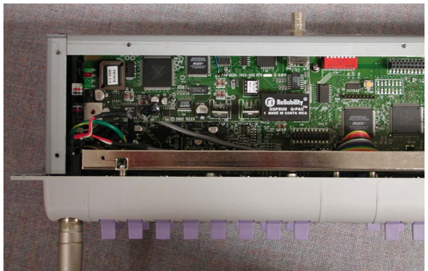
Figure 6 - View of installed CSI-100 board.
