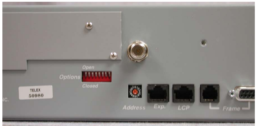
Figure 1 - CSI-100 coaxial connector location on backpanel.
