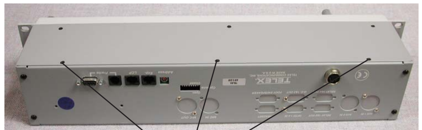
Figure 1 - CSI-100 coaxial connector location on backpanel.
