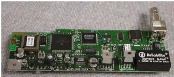
FIGURE 16. KP-32 CSI-100 coaxial system interface board
