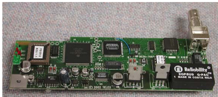
Figure 1.3 KP-32 CSI-100 coaxial system interface board.
