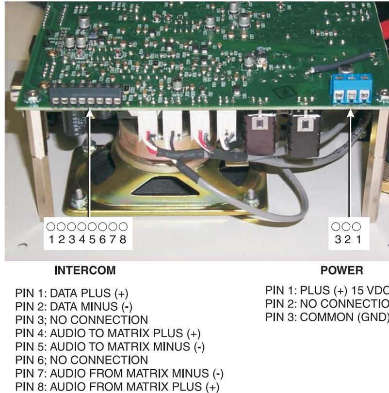
Figure 2.5 Use tie wraps to secure the cables (WKP-4 installation).
