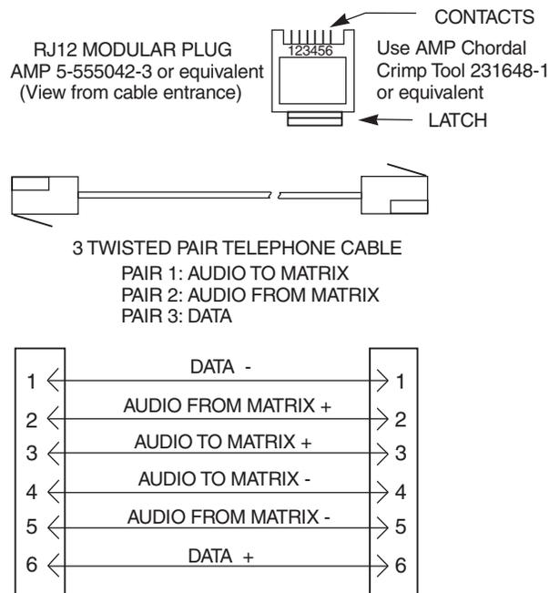
**Figure 2.3** 9-pin Intercom cable wiring diagram
