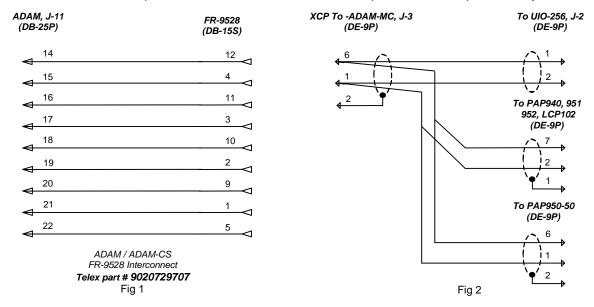
**NOTE:** If using a FR-9528 relay panel with UIO256's, the FR9528 panel will use GPI output block 1-16 in ADAMedit. GPI outs 1-8 will be active and 9-16 will not be assignable.
