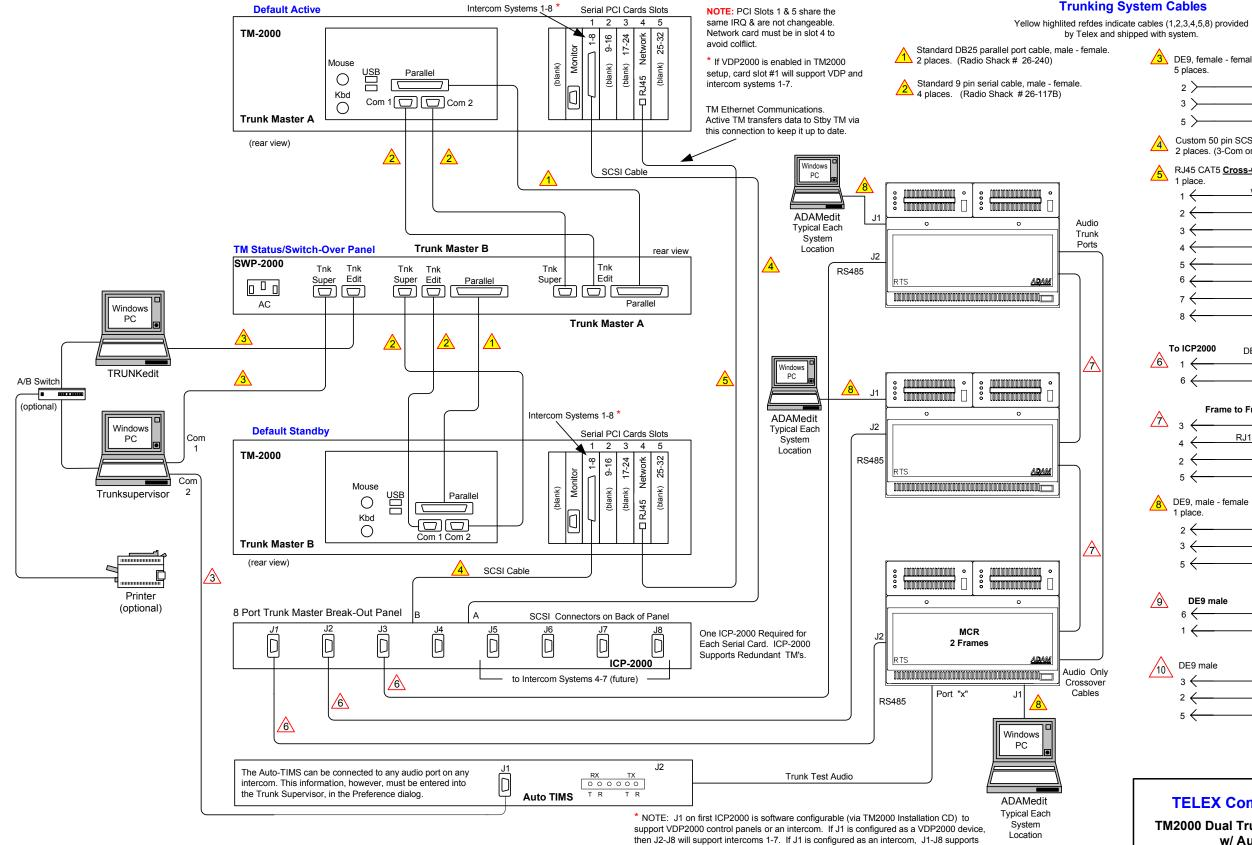
All additional ICP2000 Breakout Panels support intercoms only, no special devices.
