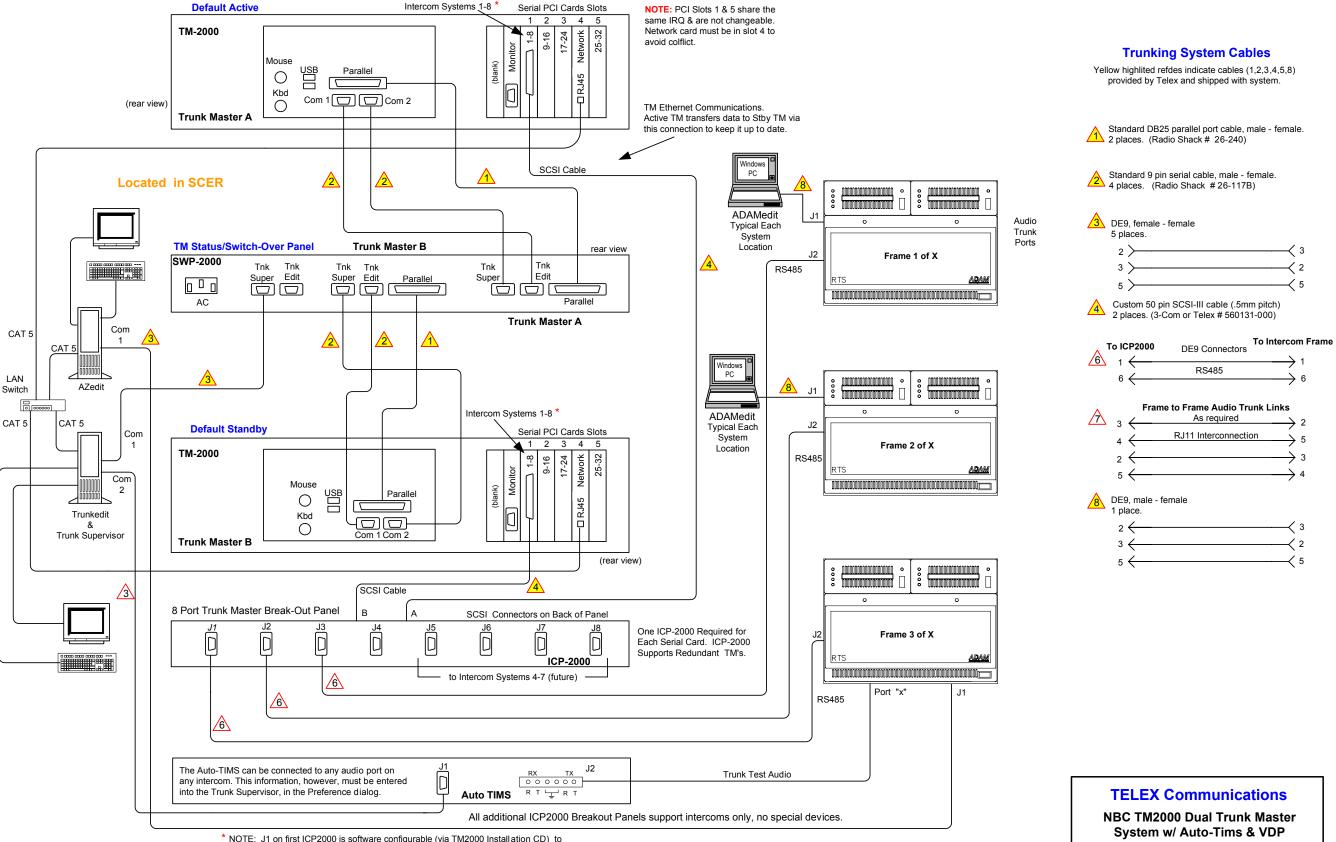
\* NOTE: J1 on first ICP2000 is software configurable (via TM2000 Installation CD) to support VDP2000 control panels or an intercom. If J1 is configured as a VDP2000 device, then J2-J8 will support intercoms 1-7. If J1 is configured as an intercom, J1-J8
