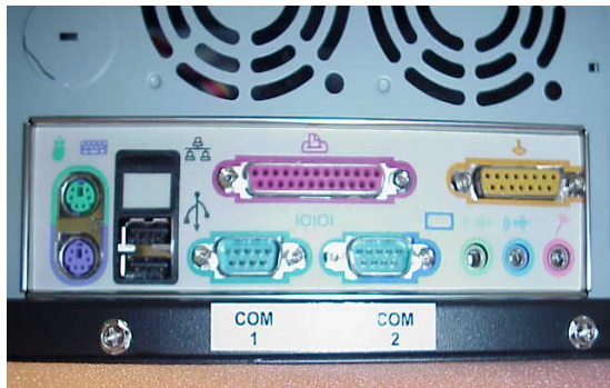
Figure 7. Serial (COM) port labels on TM-2000.
