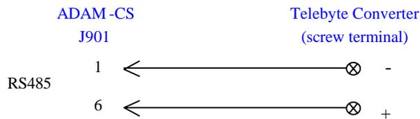
The Telebyte converter is then connected to the interface for the leased data circuit provided by the Service Provider. Pin-out provided by service provider. The data circuit must be able to pass 9.6 K baud rate minimum.
