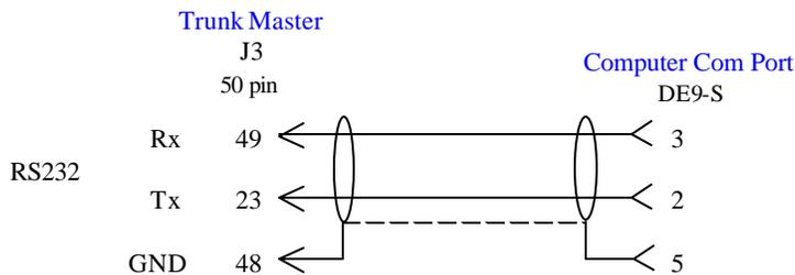
If communications with Trunk Master cannot be established, pins 2 & 3 may have to be reversed on the computer com port end.
