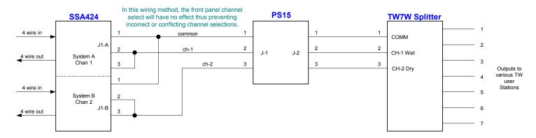
Set internal SSA Mode DIP switches to mode 1, page 16 of SSA424 User Manual.
