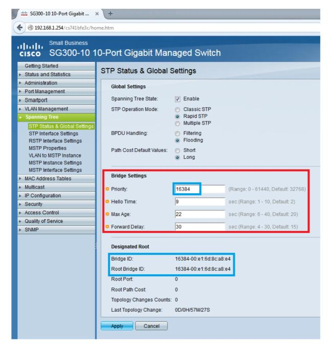
A priority value will need to be entered. Each OMNEO device has a priority value of 61440 configured so that it never becomes a root bridge. The maximum number of 20 devices for daisy chaining devices is a limitation of RSTP. You must ensure that the maximum number of hops from the Root bridge does not exceed 21.
