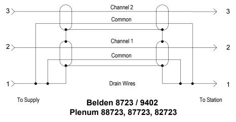
Crosstalk reduction over long distances using 2 pair individual shielded pairs
