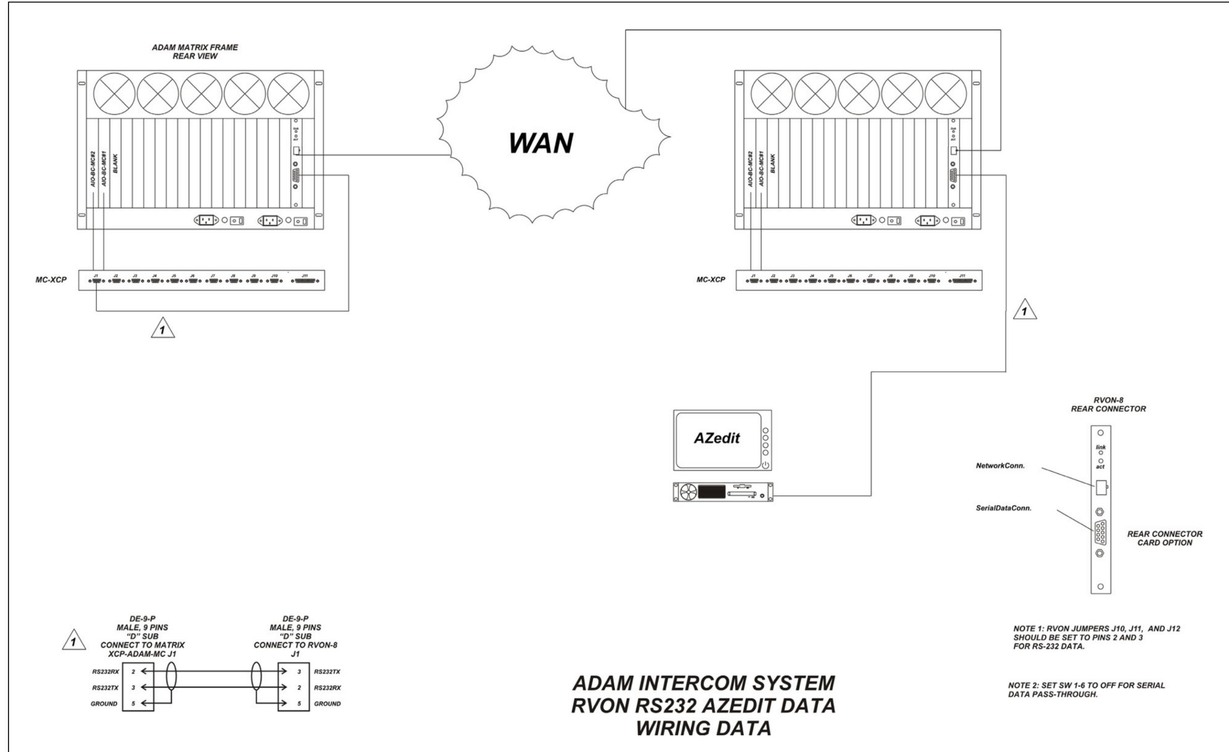
**Figure 9: CS9500 Trunking Via RVON-I/O To RVON-8**
