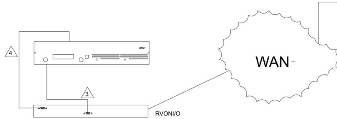
**NOTE 3:** RVON-I/O JUMPERS (J10, J11, AND J12) SHOULD BE SET TO PINS 1 AND 2 FOR RS-485 DATA
