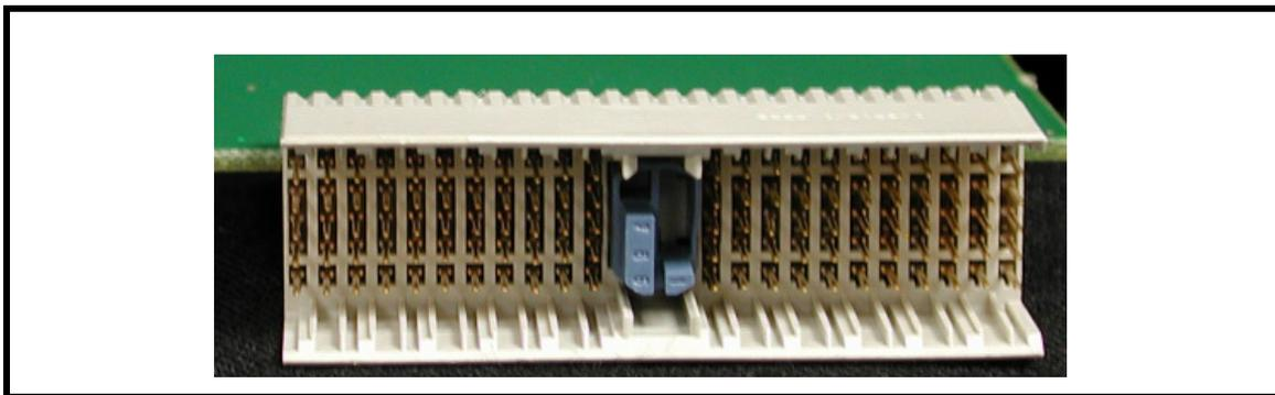
**FIGURE 3.** The RVON-16 Color Key Code. This Key Code allows only the RVON-8 or RVON-16 to plug into a blue coded, compatible backcard.
