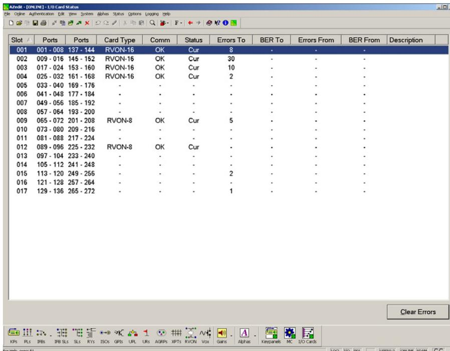
The screenshot shows the 'AZedit - [004.001] - I/O Card Status' window. It contains a table with the following columns: Slot, Ports, Card Type, Comm, Status, Errors To, BER To, Errors From, BER From, and Description. The table lists 17 slots, with slots 001-004 and 009-010 having RVON-16 cards and slots 009-010 and 012-013 having RVON-8 cards. A 'Clear Errors' button is visible at the bottom right of the table area.
