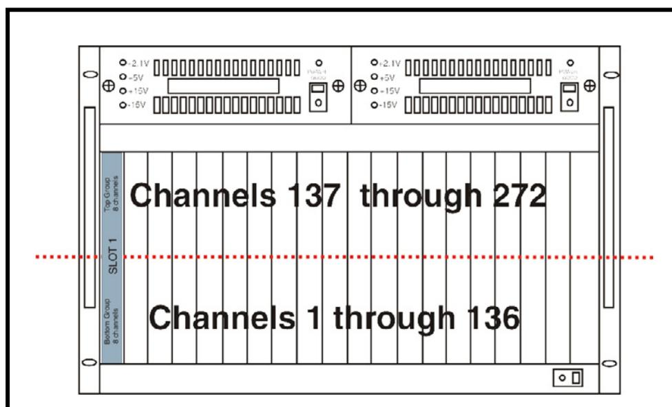
**FIGURE 1.** ADAM frame with RVON-16 cards only and the port numbering scheme
