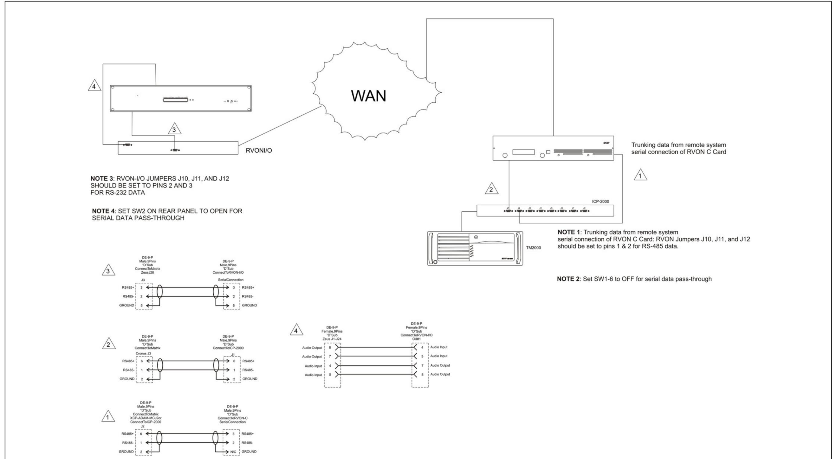
**Figure 12: Cronus Trunking Via RVON-I/O To RVON-8**
