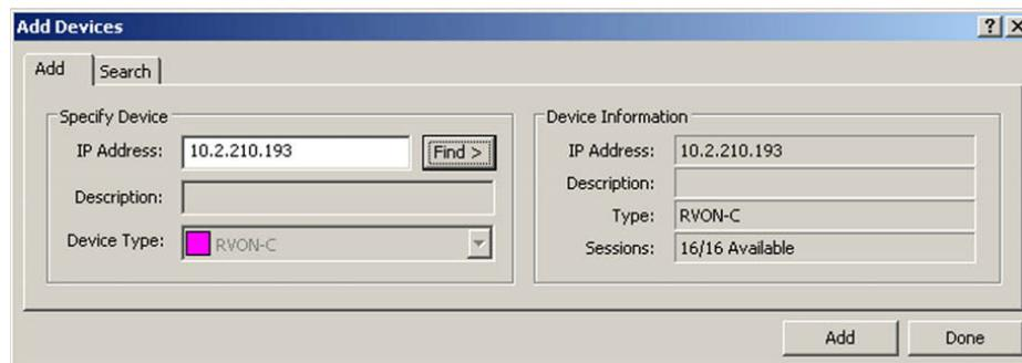
2. Under Specify device, add the **IP Address** of the device to which you want to connect.
