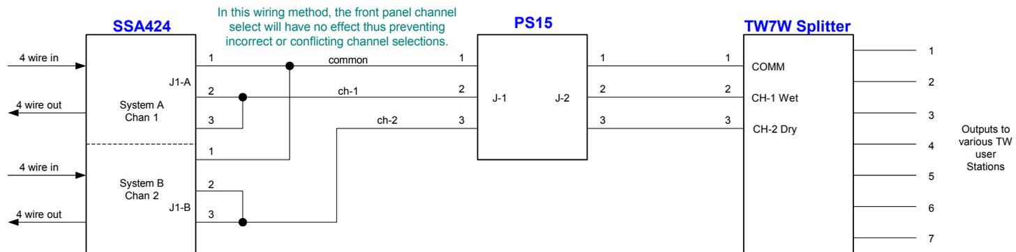
Set internal SSA Mode DIP switches to mode 1, page 16 of SSA424 User Manual.
