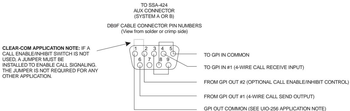
**UIO-256 APPLICATION NOTE:** GPI OUT - AT THE UIO-256 END, USE THE NORMAL OPEN (NO) CONTACT FOR GPI OUT CONNECTION, AND USE THE RELAY COMMON CONTACT FOR THE COMMON CONNECTION.
