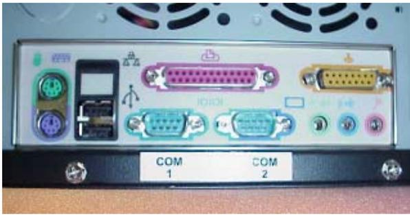
**Figure 7 - Serial (COM) port labels on TM-2000.**
