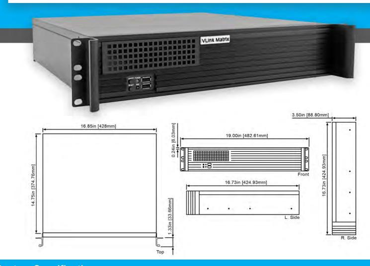
System Specifications: Form factor: 19" 2U Short Depth (15.4") Rackmount Processor: Intel core i7-8700 (Up to 4.6GHz) Storage: 250GB SSD Memory: 8GB DDR4 LAN: Onboard Gigabit LAN; 2-Port Ethernet Adapter Card
