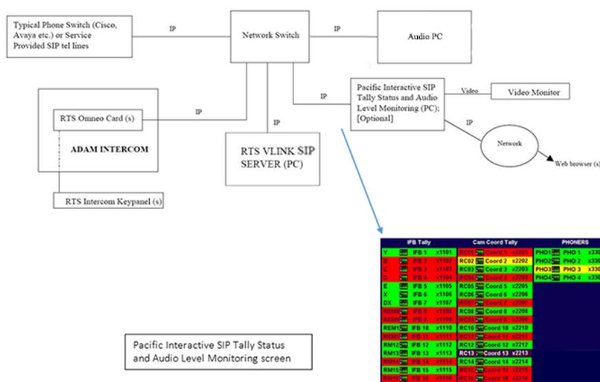
**FIGURE 1.** RTS SIP Interface Solution (Dante) Block Diagram
