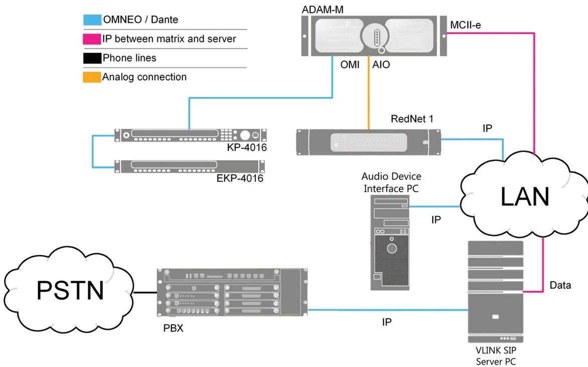
**FIGURE 3.** SIP Server via analog, using RedNet 1 box
