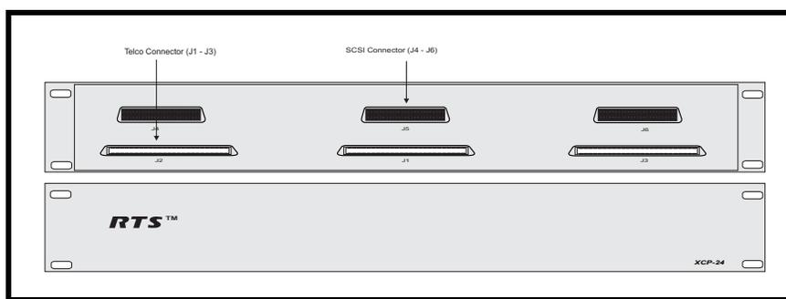
The XCP-24-USOC Breakout Panel allows for the expansion of the ADAM frame using Telco connectors. When using the XCP-24-USOC breakout panel, you **MUST** use the SCSI backcard with the AIO-16 card
