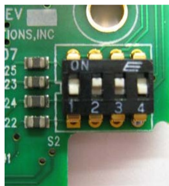
FIGURE 10. Use this switch setting scheme for RTS Standard Cable (USOC).
