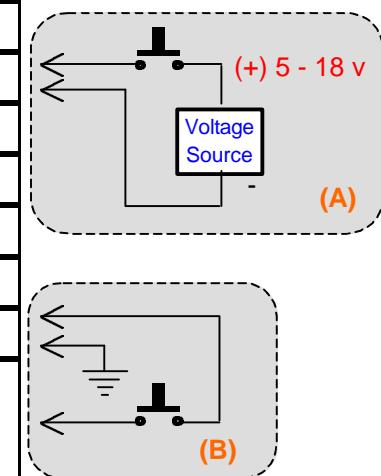
Example "A" shows interconnection of external control voltage source. Example "B" shows control via internal 18 volt source.
