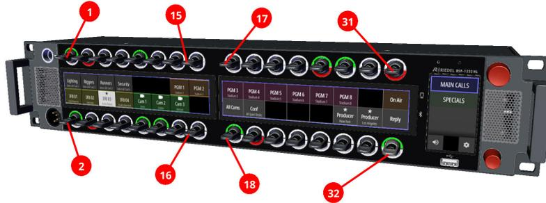
figure 9: Numbering of lever keys
