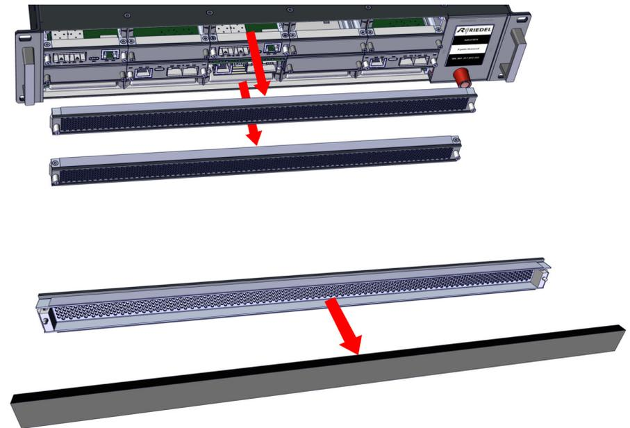
figure 18: replacing front filter
