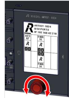
Turning the rotary encoder
