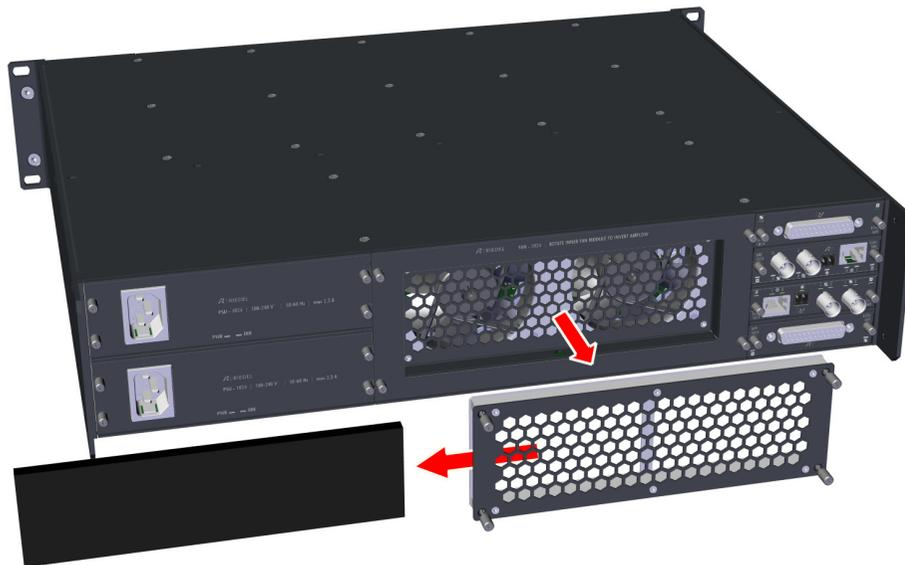
figure 19: replacing rear filter
