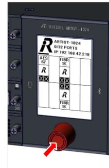
Pushing the rotary encoder
