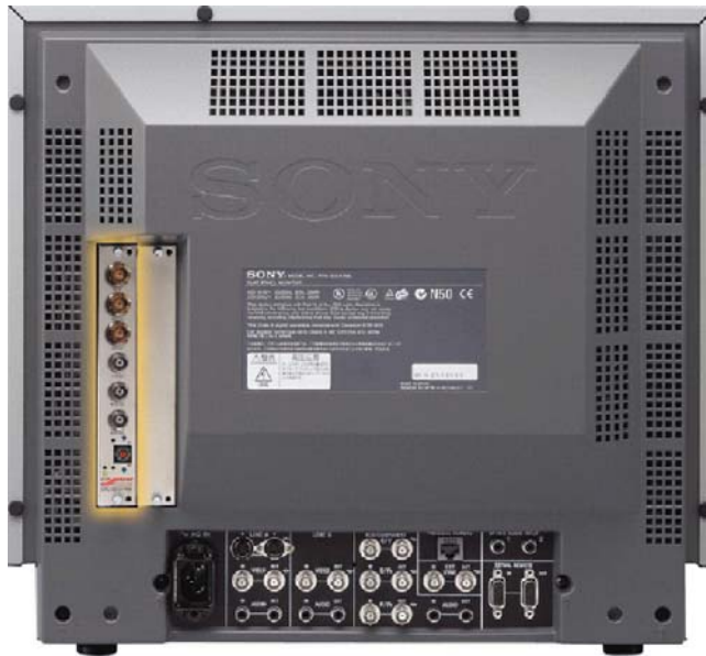
Figure 2. DAC-9213-PVM installed in Sony PVM/BVM monitor - rear view
