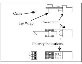
Once the cables have been wired, install the connectors according to the illustration below.
