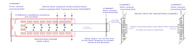
A) The rear support bars can be attached to the Ross frame in six possible positions. See the illustration. Choose the position that suits the cabinet depth and will give approximately a 1/2 inch projection beyond the previously mounted bracket. Using four screw per bracket as shown in the illustration, attach both bars.
