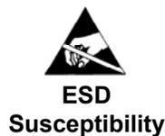
Static discharge can cause serious damage to sensitive semiconductor devices. Avoid handling circuit boards in high static environments such as carpeted areas, and when wearing synthetic fiber clothing. Always exercise proper grounding precautions when working on circuit boards and related equipment.
