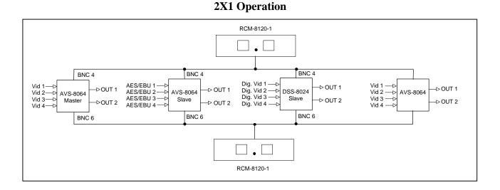
In the above diagram, the RCM-8120-1 module connected to BNC 4 will control crosspoint 1 on each utility switch. The RCM-8120-1 module connected to BNC 6 will control crosspoint 2 on each utility switch.
