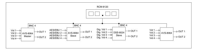
In 4X1 operation, switch 2 on each card is set to follow switch 1 (via JP6 SW2 CONTROL being put into the FW 1 position). Therefore, both crosspoints on each card select the same input. The jumpers are set as follows:
