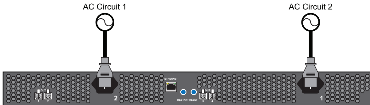
Figure 4.5 Ultripower — Power Connections
