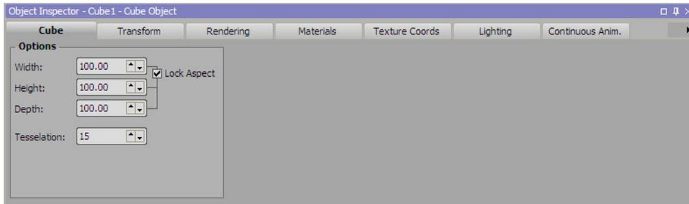
4. In the **Options** section, use the **Width** box to enter or select a value in pixels to set the width of the cube object.
