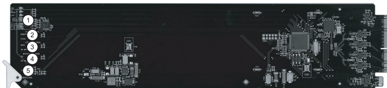
Figure 3.1 Card-edge Controls (SRA-8601A shown)
