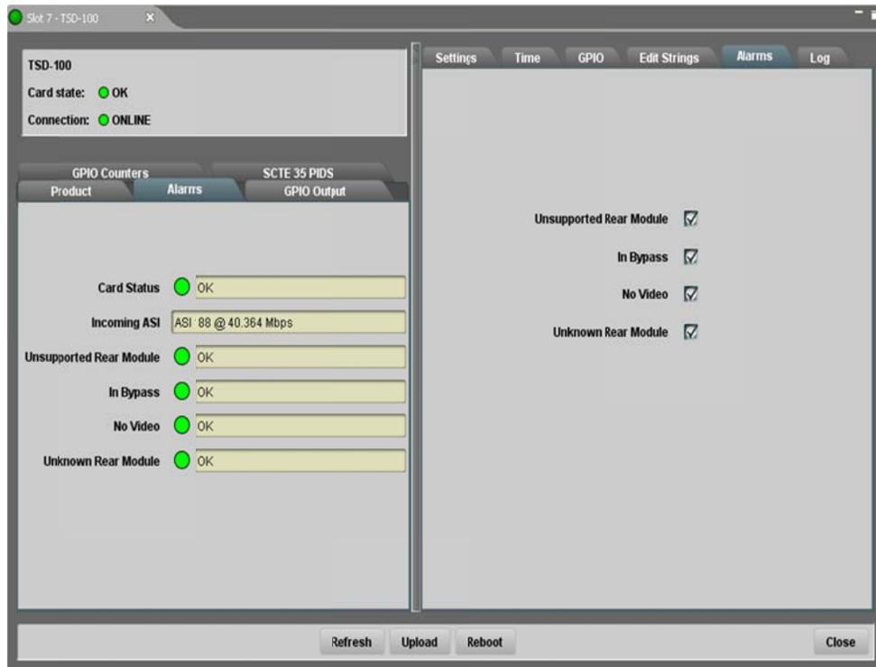
The alarm conditions listed in the Alarms status screen are qualified by the selections made on the Alarms setup screen, which is on the right side of Figure 9. Any error conditions that are checked on the Alarms setup screen will cause the Card Status to turn red when they occur. Alarm conditions that are unchecked will be ignored in compiling the Card Status.
