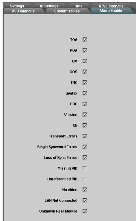
Figure 23. Alarm Enable menu
