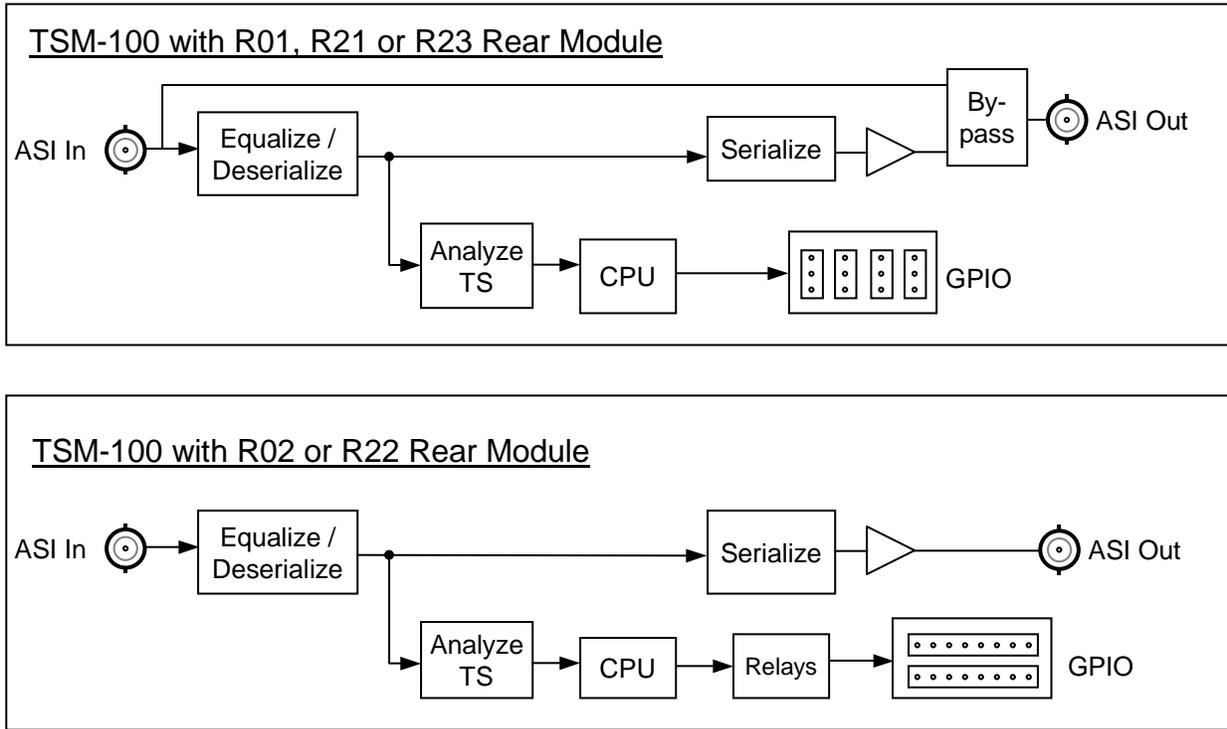
Figure 1. Simplified Block Diagrams of TSM-100 Functions
