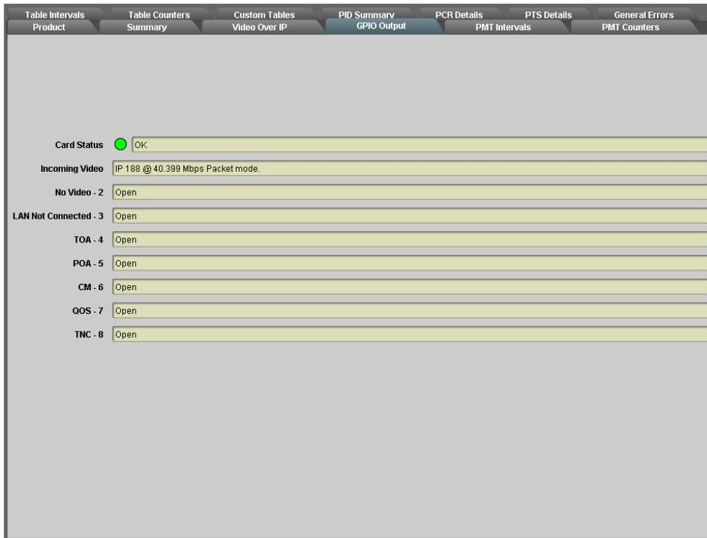
Figure 19: GPIO Output Status
