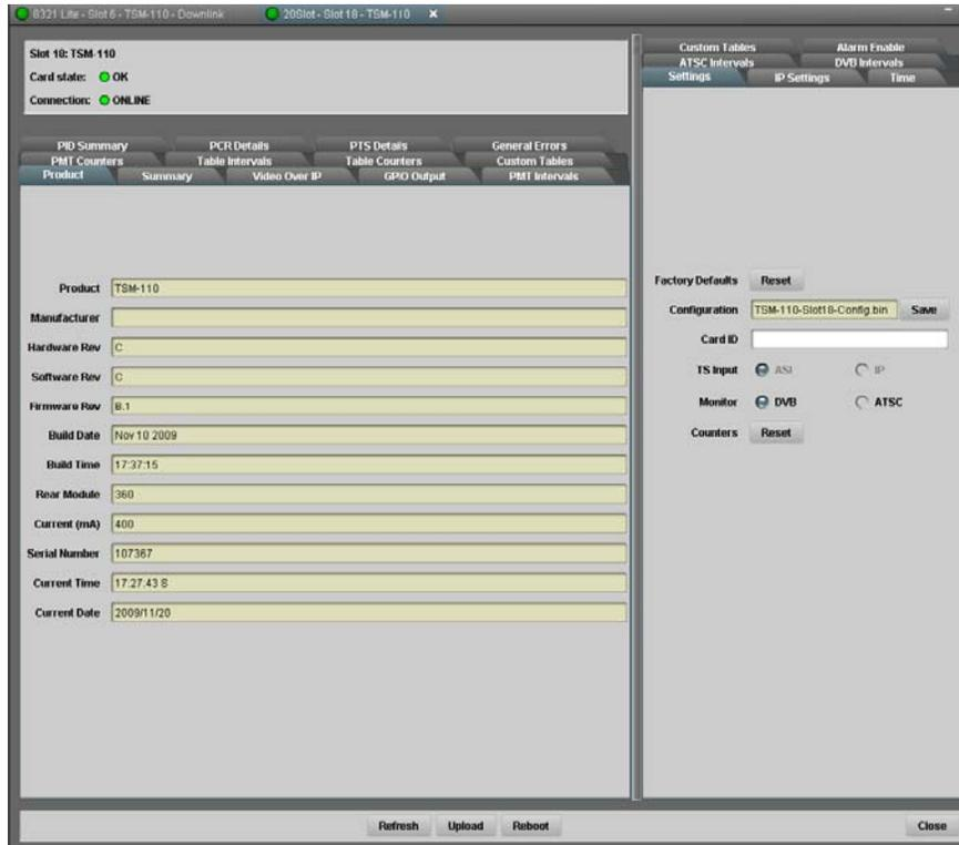
Figure 5: TSM-100 Dashboard Screen, showing Product Status and Settings
