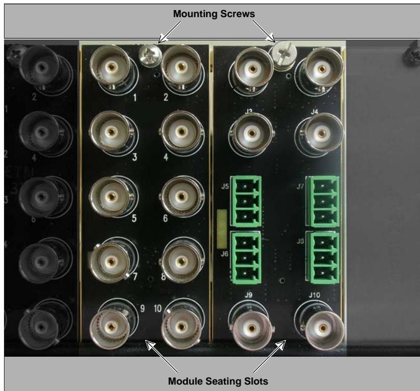
**Figure 2: Rear Module Installation, showing R1-10B (left) and ONG-MDL-R01 (right) modules**
