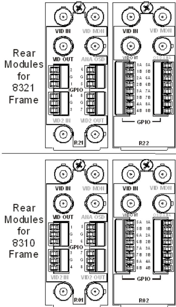
Figure 3. Top, left to right: ONG-MDL-R21, R22 and R23; Bottom, left to right: ONG-MDL-R01 and R02
