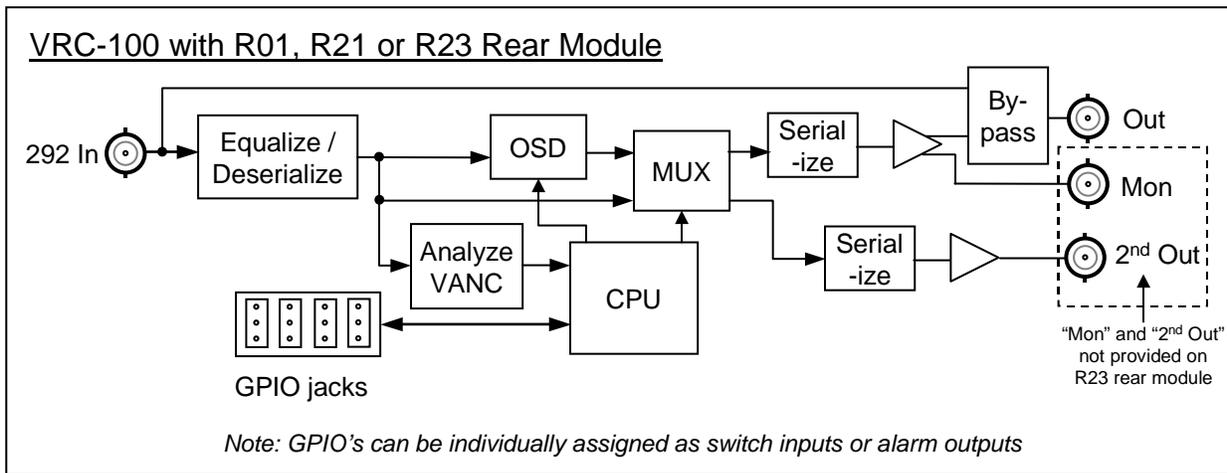
Figure 1. Simplified Block Diagrams of VRC-100 Functions
