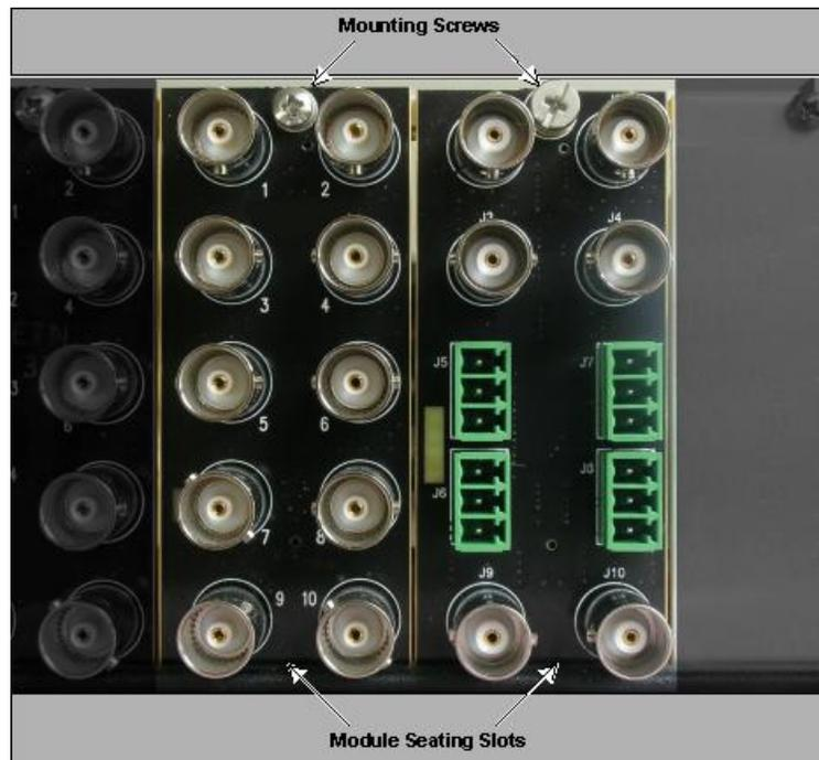
Figure 2: Rear Module Installation, showing RM-8300-B (left) and ONG-MDL-R01 (right) modules
