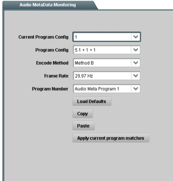
Figure 17. Audio Metadata Monitoring – main sub-tab
