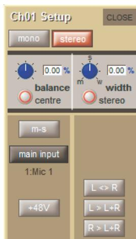
In addition to the standard routing button, stereo channels also have an **m-s** button which switches in a decode function for replaying M-S signals as a normal stereo pair. There are three further buttons in this panel: **L<>R** swaps the channel's left and right outputs, **L>L+R** sends the left signal to both left and right busses, and **R>L+R** sends the right signal to both left and right busses.
