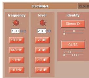
The frequency of the oscillator is controlled by the left-hand **frequency** pot, and its audio level is controlled by the right-hand **level** pot. The buttons below each pot, can be used to set the oscillator to standard frequencies (**100Hz, 440Hz, 1kHz, 10kHz**) and levels (**-3dB, -6dB, -12dB, -18dB**). The current value of each parameter is displayed below its pot.
