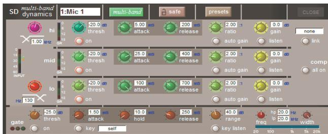
Each band provides the same controls as the single-band module, with global controls for on/off and link functions. Each band can also be switched on and off individually.
