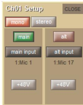
The inputs available on an Input channel include feeds from the external IO racks, the local inputs on the back of the console and a variety of internal signals. Pressing either the **main input** or **alt input** routing button in the **Setup** display opens the **Input Route** display. The signal feeding each input can then be selected as described in the Getting Started section of this manual.
