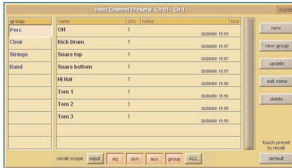
**Note that presets are specific to a channel type: The Presets display will only list those presets which apply to the current channel type.**
