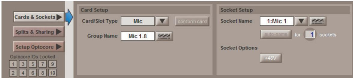
A range of sockets can be named with the same label and an incrementing number by using the **auto-name** function below the **Socket Name** box:
