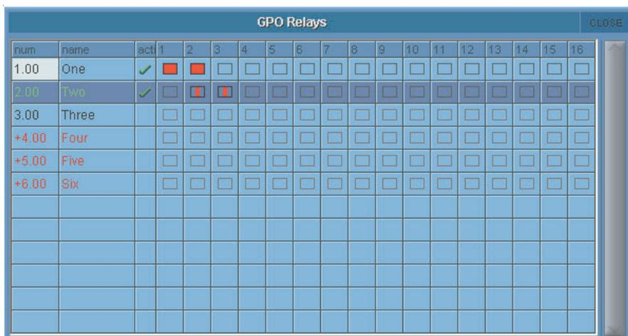
The GPOs are displayed in columns and the Snapshots in rows. Selecting a box will cause it to go red, indicating that the relay will open with that Snapshot and close with the following Snapshot.
