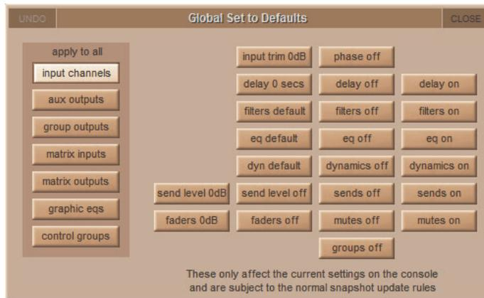
The **Global Set to Defaults** Panel allows global default settings to be applied to the console. Select the Channel type from the list on the left side of the panel, and then select the operation to perform from the available functions. The **UNDO** button in the top left-hand corner undoes all changes since the panel was opened.
