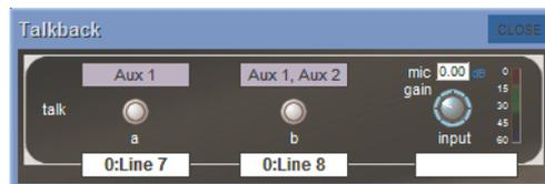
The white boxes across the bottom of the display open routing panels, allowing for selection of the main output for each talk buss, and the **input** used for the talkback mic, using the standard routing procedure. Routes can also be named in the normal way. The current routes are displayed in the boxes. Note that multiple outputs can be selected (though only the first is displayed) and there is an alt input available.
