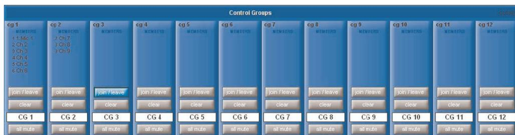
This display consists of basic versions of each Control Group channel strip, including the channel assignments lists and a number of basic settings which can also be adjusted in the display: **join/leave**, **clear** and **all mute**. The Control Group naming controls are also available within the display's channel strips.
