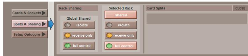
Normally, the input gain, phantom power and pad of each DiGiRack input is controlled remotely from the SD10. However, in multi-console systems where DiGiRacks are connected with MAD1 and shared between two DiGiCo consoles, only one of the consoles can remotely control these rack settings. Therefore, the level of control given to each console must be defined. There are three levels of control: **isolate**, **receive only** or **full control**.
