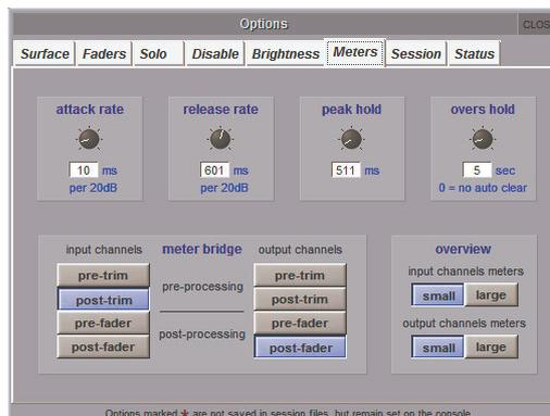
The four pots across the top half of the display affect the attack and release reaction time (**attack rate** and **release rate**), the **peak hold** time and the **overs hold** time. The current setting for each is displayed in either milliseconds or seconds, below each pot. Touching each pot assigns it to the Touch-Turn encoder.
