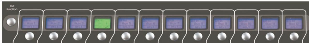
When the **lcd function** button is pressed, the Channel Select buttons beneath the LCD displays are used to activate the various functions and to select channels as required:
