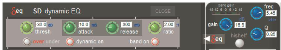
Switch the EQ band on and off using the **band on** button, and activate the band's dynamics using the **dynamic on** button.
