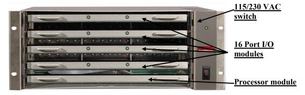
*Note:* The 4 RU RS-422 64 port system can consist of up to four 16 port I/O modules and a control processor. The 4 RU 64 port frame can be configured as a 16, 32, or 64 port router. It can be expanded in 16 port increments to a maximum of 64 ports by just adding I/O modules.
