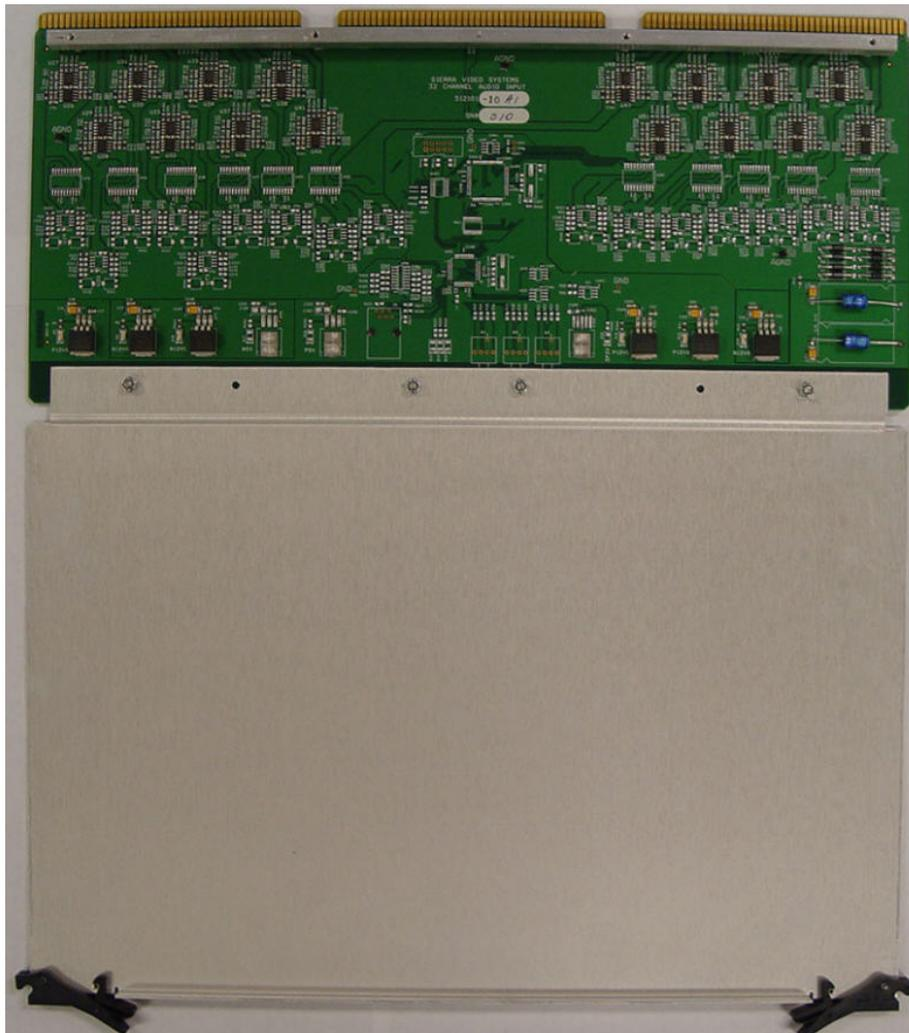
The output of the input buffer circuits are connected to the switching matrix via the internal motherboard. The 64x64 frame has positions for two 32-channel buffer modules; and the 128x128 frame has positions for four 32-channel buffer modules.
