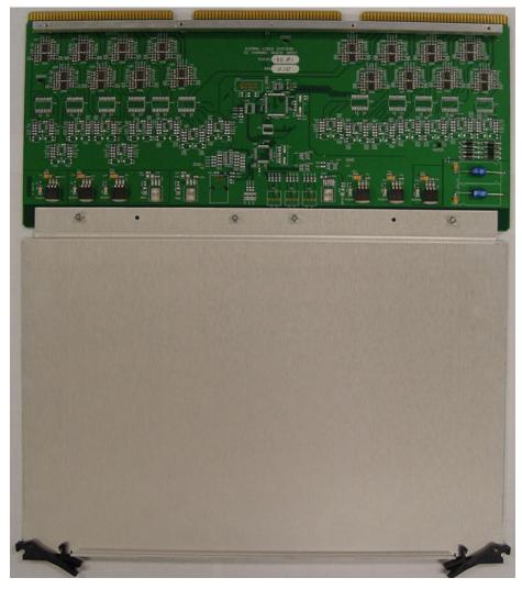
The output of the input buffer circuits are connected to the switching matrix via the internal motherboard. The 64x64 frame has positions for two 32-channel buffer modules; and the 128x128 frame has positions for four 32-channel buffer modules.
