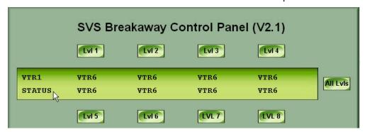
"Programmable Control Panel" adds 8x8 programmable XY buttons for single-button takes.
