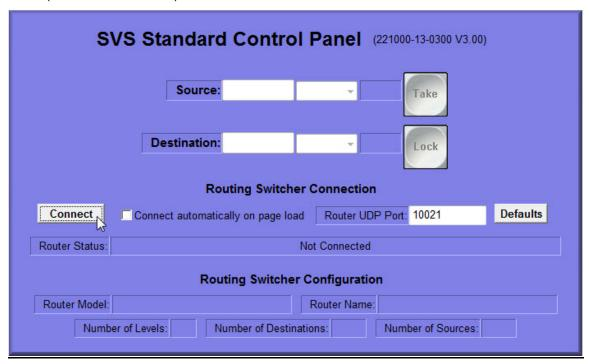
Click on **Connect**. The message "Getting Router Model" will display next to **Router Status**. This is an indication that the program is attempting to contact the router for information.
