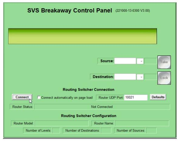
Click on **Connect**. The message "Getting Router Model" will display next to **Router Status**. This is an indication that the program is attempting to contact the router for information.
