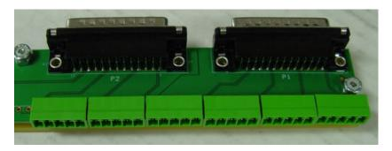
The 25-pin "D" connectors each support a group of 4 inputs or outputs and the screw terminals are in groups of 4 containing 2 inputs or outputs each.
