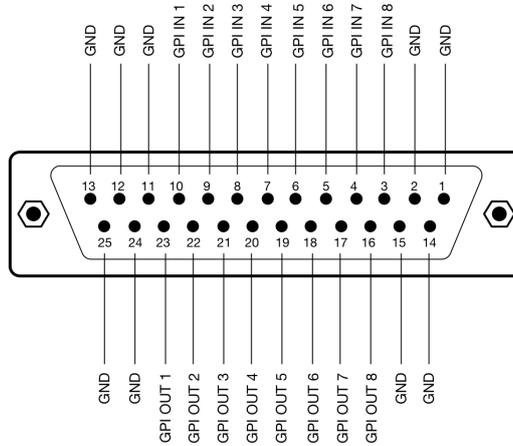
This is the pinout for the DB25 Connector we use on the SDI-GPI Link:
