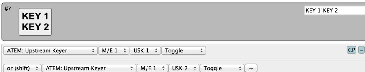
This is how the button “KEY1 / KEY2” is configured in the web interface. As it appears, this button will toggle upstream keyer 1 or 2 on an ATEM switcher depending on whether the controller is in shift-state or not.
