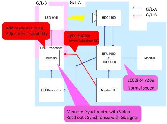
LED processor needs delay adjustment to move out banding to outside picture. If the banding is acceptable level then it is not required
