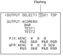
2 Turn the CONTROL knob to change the displayed page to the desired page, then press the CONTROL knob.
