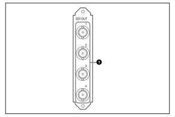
SDI OUT 1, 2, 3, 4 (3G/HD serial digital interface output 1-4) connectors (BNC-type)
