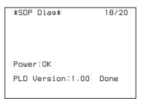
**Power:** Status of power supply to the SDP board **PLD Version:** SDP board PLD version
