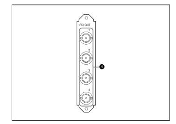
SDI OUT 1, 2, 3, 4 (3G/HD serial digital interface output 1-4) connectors (BNC-type)
