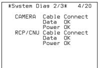
CAMERA Cable: Camera cable connection status CAMERA Data: Camera data transmission status CAMERA Power: Camera power supply status RCP/CNU Cable: This unit's REMOTE connector cable connection status
