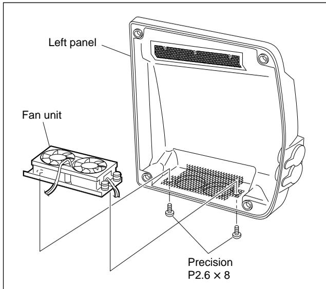
3. Remove the three screws of the fan holder, and remove the fan holder.
