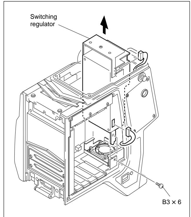
6. Attach the new switching regulator in the reverse order of steps 1 to 5.
