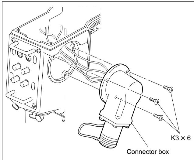
6. Remove the four screws, and remove the CCU connector.
