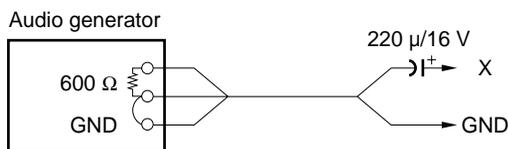
5. Test point: Pin 61/EX-464 board
