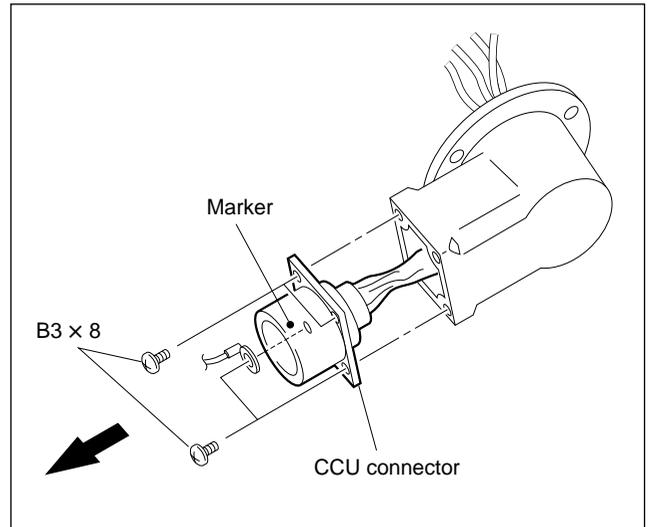
7. Attach the new CCU connector in the reverse order of steps 1 to 6.
