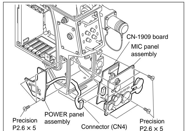
6. Remove the four screws in front of the chassis assembly and two screws of the board rail, and remove the board rail from the right side.
