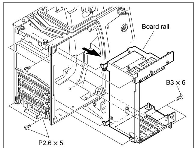
7. Remove the two screws in front of the chassis assembly, and remove the CN-1705 board and CN-1735 board.
