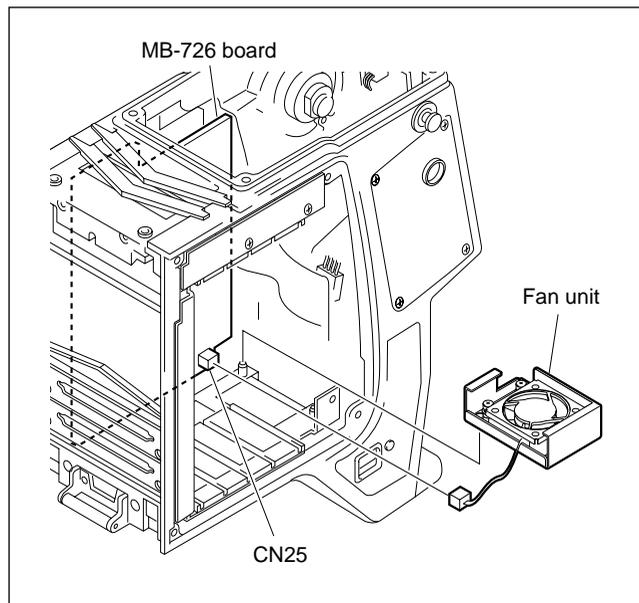
3. Remove the three screws of the fan holder, and remove the fan holder.
