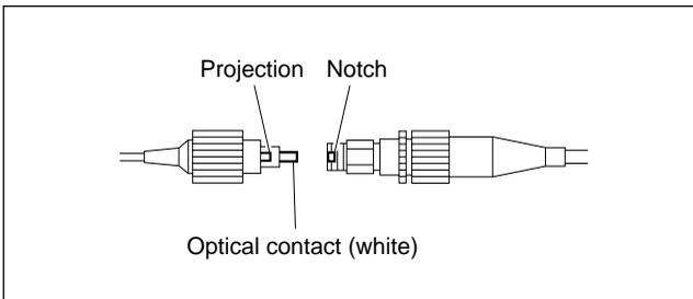
**2-6. Replacing the CCU Connector**
