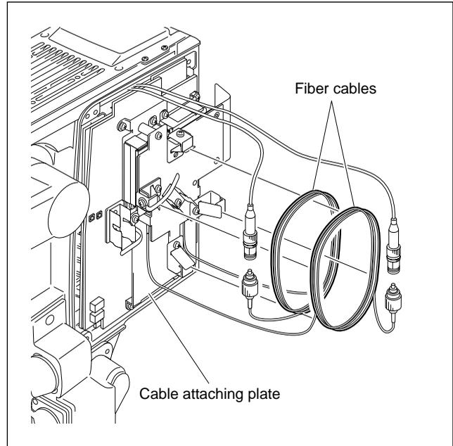
4. Remove the three screws shown in the figure, and remove the cable attaching plate.
