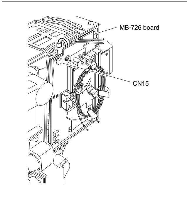
5. Remove the three screws, and remove the connector box.
