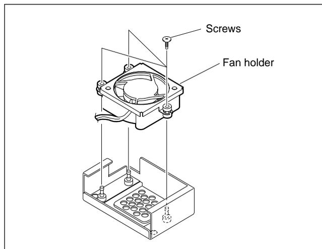
4. Remove the two screws securing the fan, and remove the fan.
