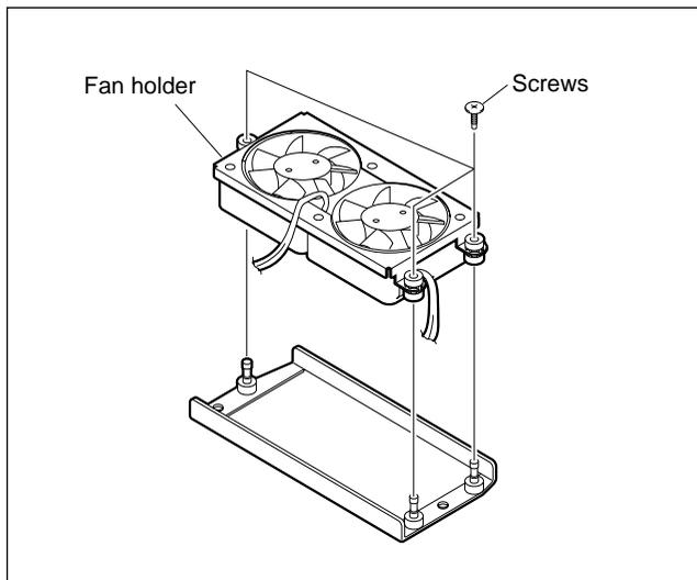
4. Remove the two screws securing each of the two fans, and remove the two fans.
