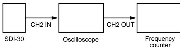
1. Connect the oscilloscope and the frequency counter as shown in the figure.
