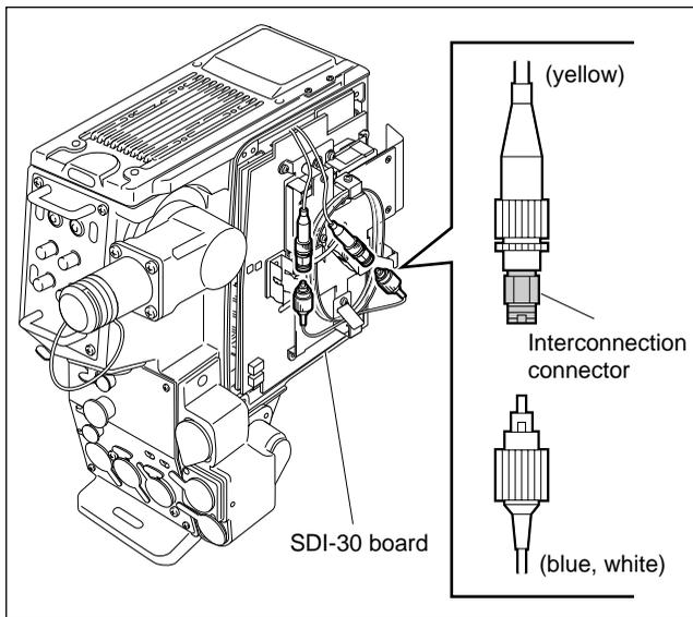
3. Disconnect the fiber cable wound around the cable attaching plate.
