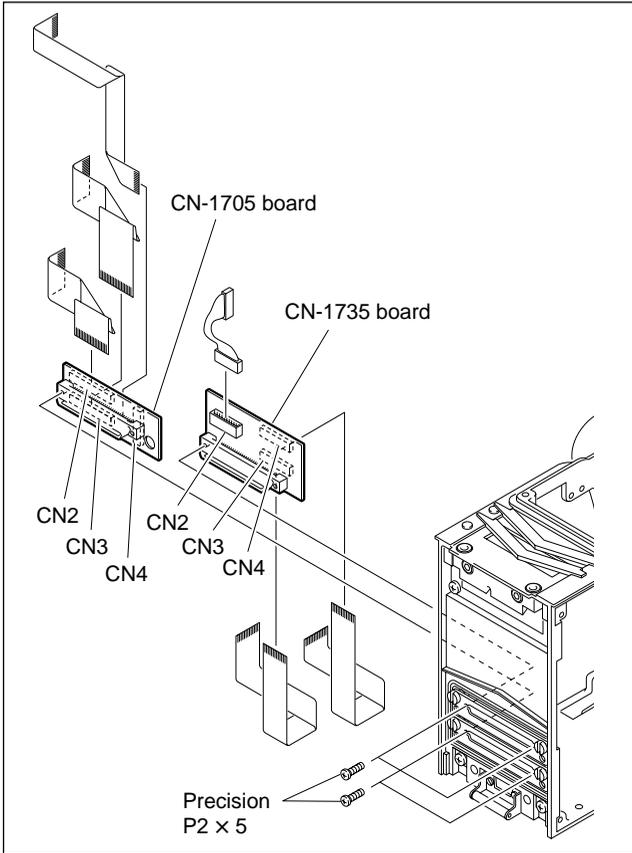
10. Attach the new 68P connector in the reverse order of steps 1 to 9.
