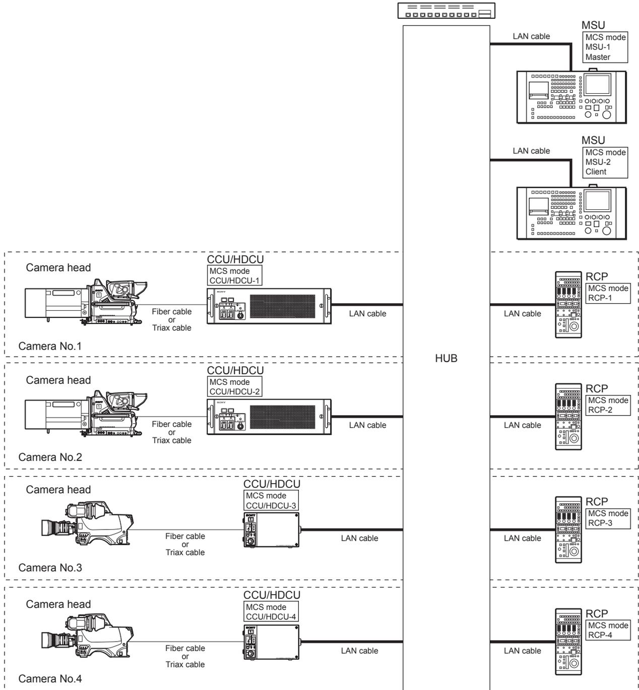
( The power to the RCP should be supplied ( via PoE HUB or to the EXT I/O connector. )
