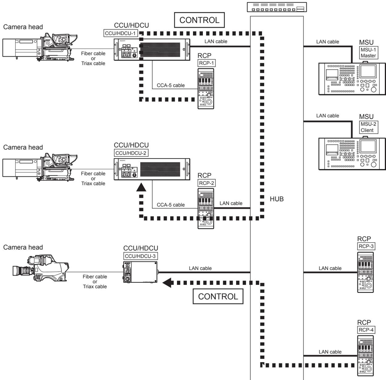
The RCP assignment is also possible in the system using the CNU. However, because the RCP assignment is possible for only the equipment that is connected to the same CNU, combination is restricted in the system using more than 12 units. We can get rid of such restriction by setting the network connection.
