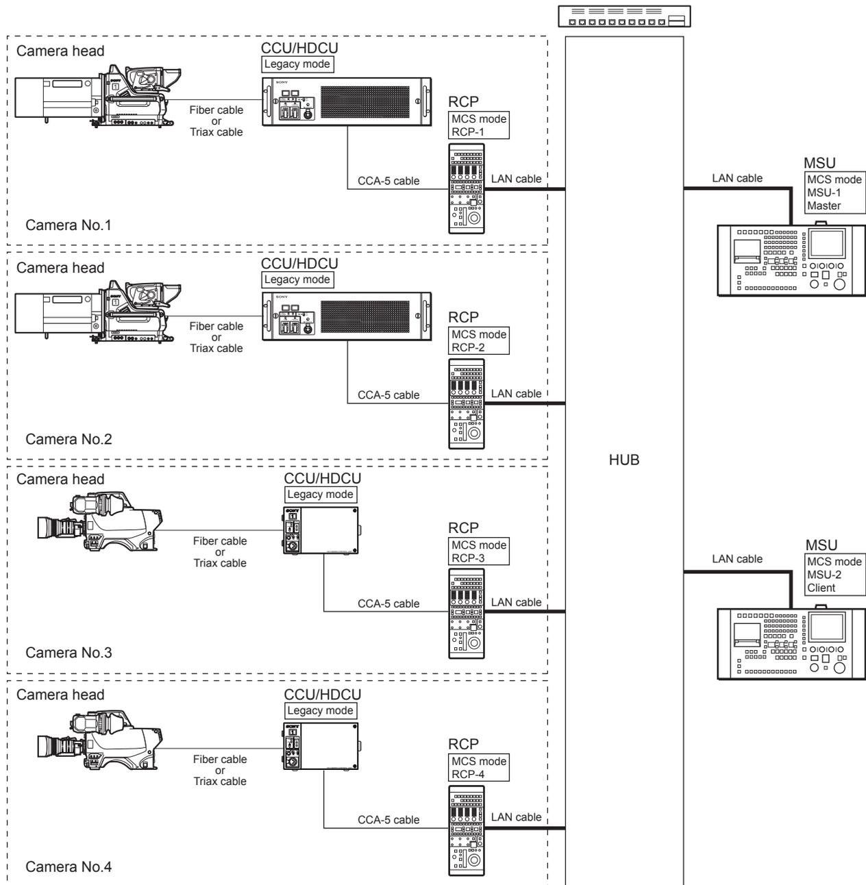
(When the HUB does not support PoE, the power to the RCP is supplied from CCU/HDCU via CCA-5 cable. When the HUB supporting PoE is used, or when the power is supplied to the EXT I/O connector, the RCP can operate even when the power to the CCU/HDCU is shut down. If the power is supplied from both sources, the power of higher voltage has priority.)
