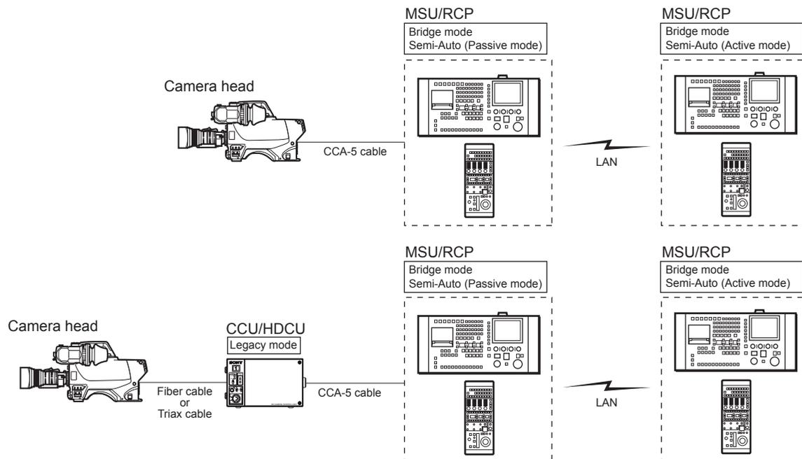
( Even when the HUB does not support PoE, the power to the RCP is supplied from CCU/HDCU via CCA-5 cable. If the power is supplied from both sources, the power of higher voltage has priority. )
