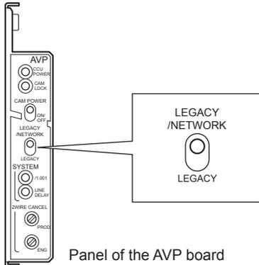
When this switch is used, switching between the network connection and the Legacy mode becomes possible from the panel. It helps us when the communication mode should be switched in an emergency.
