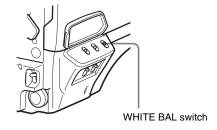
2 Select the filter setting according to the lighting conditions.
