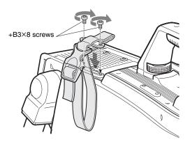
4 ① Release the buckle, ② bundle the cable with the belt, ③ then lock the buckle again.
