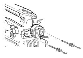
Using the two bolts (M4  $\times$  8) and the washers removed from the camera in step 2, attach the rotation mechanism assembly of the BKW-401 to the camera.
