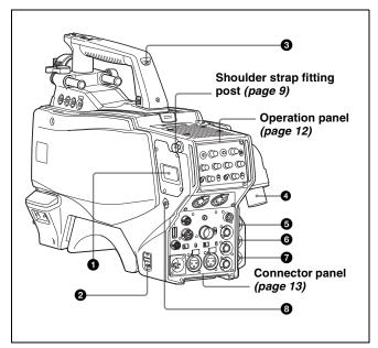
**DC power supply out connector (2-pin)** Supplies power to an external device up to 2.5 A.
