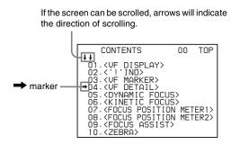
Turn the MENU SEL knob/ENTER button to align the arrow marker ( $\rightarrow$ ) to the page to be set and press the MENU SEL knob/ENTER button.
