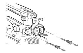
**3** Using the two bolts (M4×8) and the washers removed from the camera in step 2, attach the rotation mechanism assembly of the BKW-401 to the camera.
