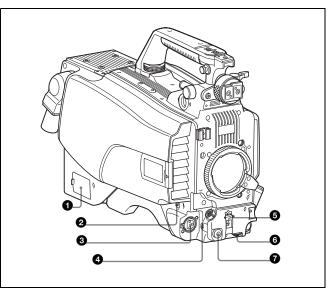
**1** NETWORK TRUNK connector (RJ-45 8-pin) Connects a device connected to the CCU's NETWORK TRUNK connector to the network.
