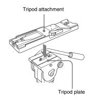
2 Place the camera on the tripod attachment, and slide forward it along the groove of the tripod attachment until it clicks.
