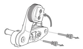
2 In the same manner as step 1, remove the viewfinder shoe of the camera from the front-rear positioning mechanism assembly.
